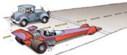
Suppose both of these vehicles, starting from rest, speed up to 60 km/h. They will have the same change in velocity, but, since the dragster can get to 60 km/h faster than the old car, the dragster will have a greater acceleration.
